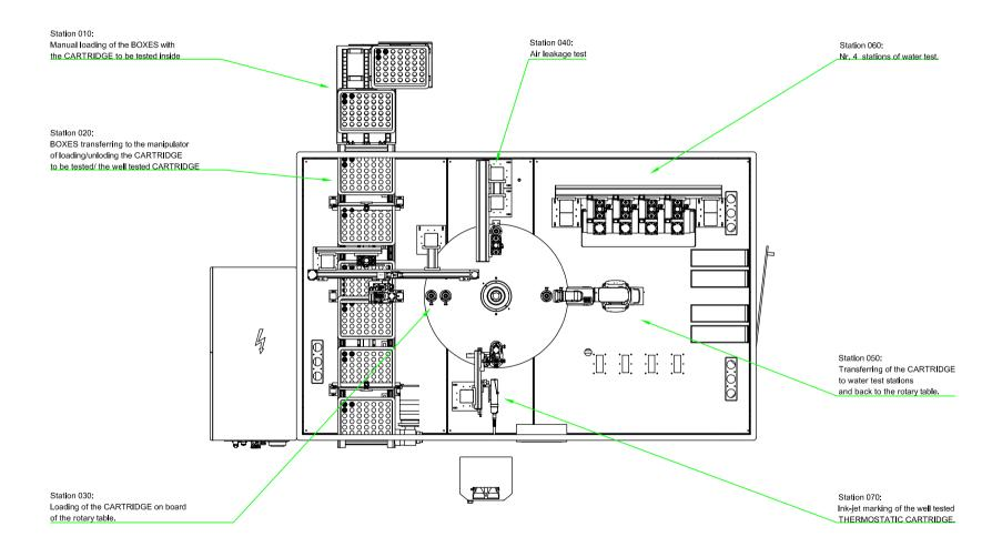
THERMOSTATIC CARTRIDGES TEST BENCH
